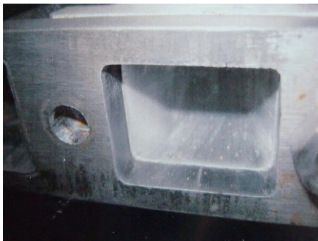
Smooth passage through manifolds
