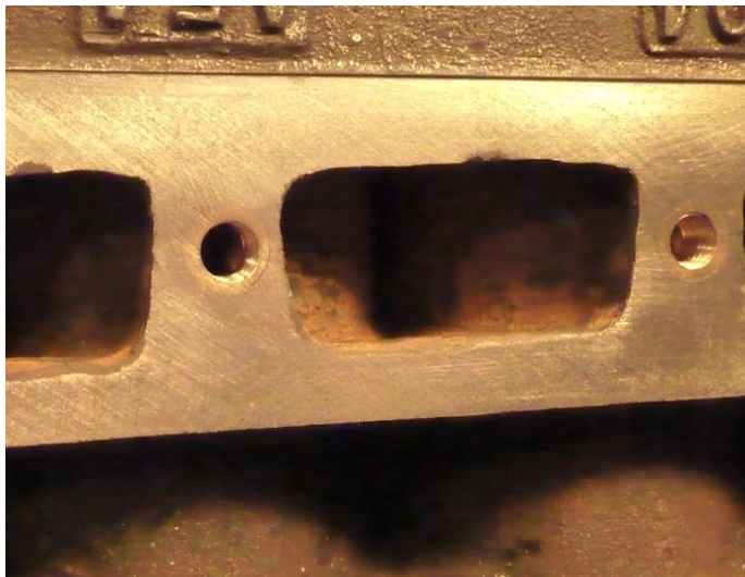
New bushes finished flush
