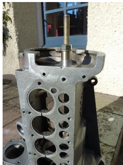
Extractor in position
