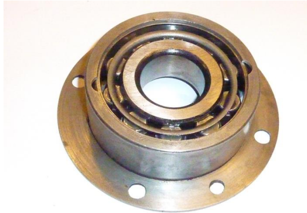
Rear main- showing housing cut-outs
