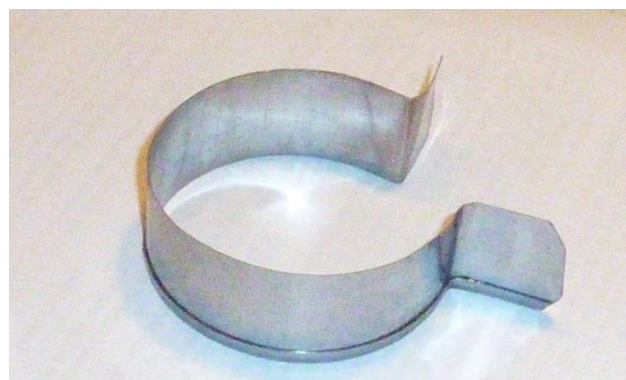
Improvised piston ring clamp
