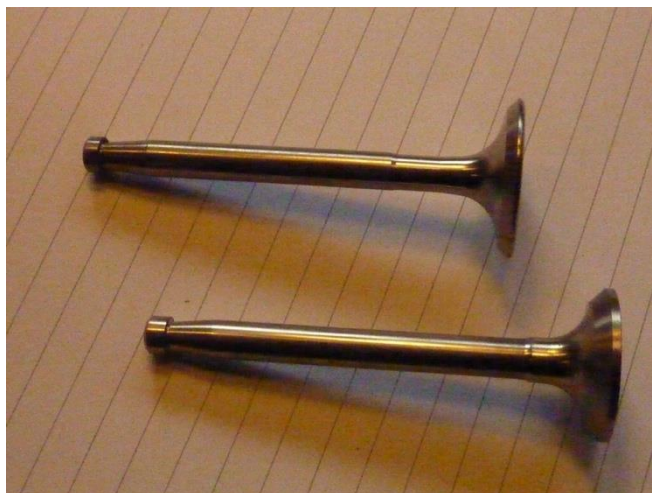
Inlet (top) and exhaust valves
