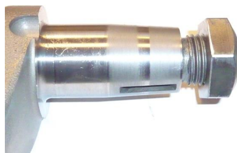
Matching crankshaft taper
