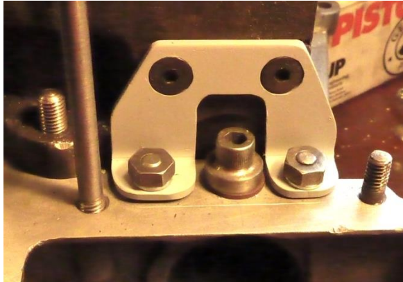
Front - straddles the cam bearing screw
