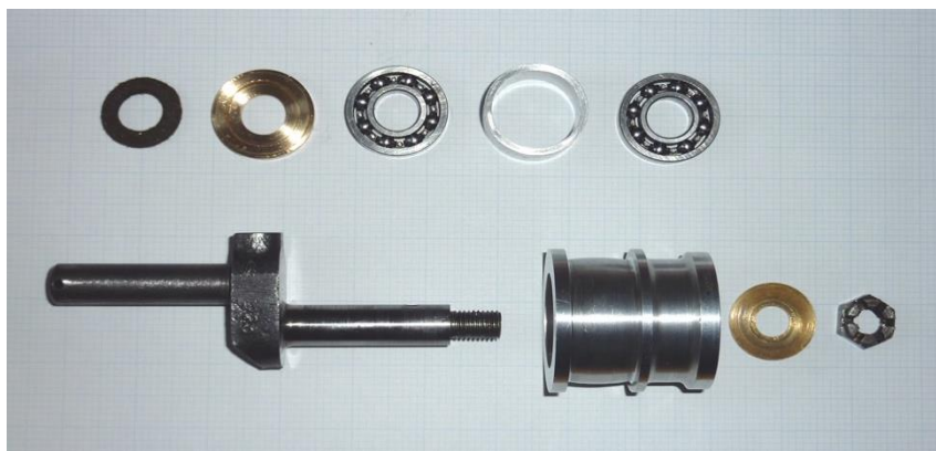
Spindle & components ready for assembly
