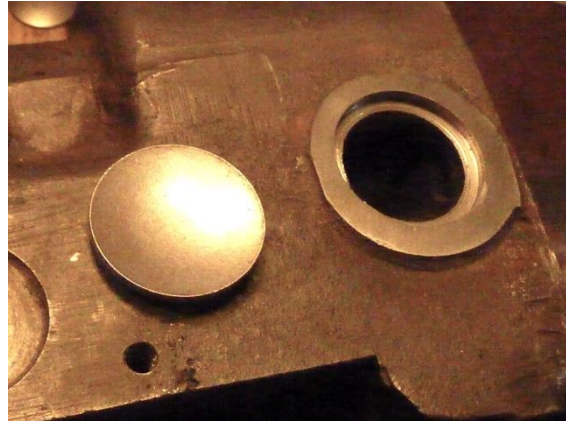
New core plug and clean seating
