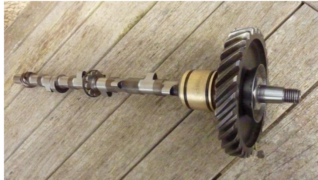
Camshaft assembly ready for insertion
