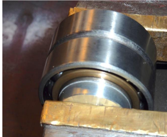
Assembly held for checking pre-load
