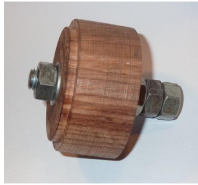
Jig to ensure ring is concentric
