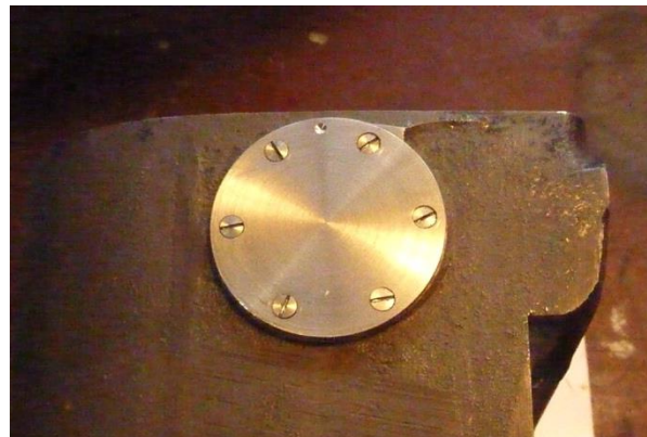
Core plug cover plate complete
