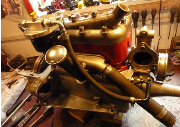
Full flow oil filter - return connection
