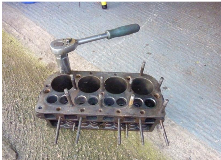
Using a 'roller cage' type stud extractor
