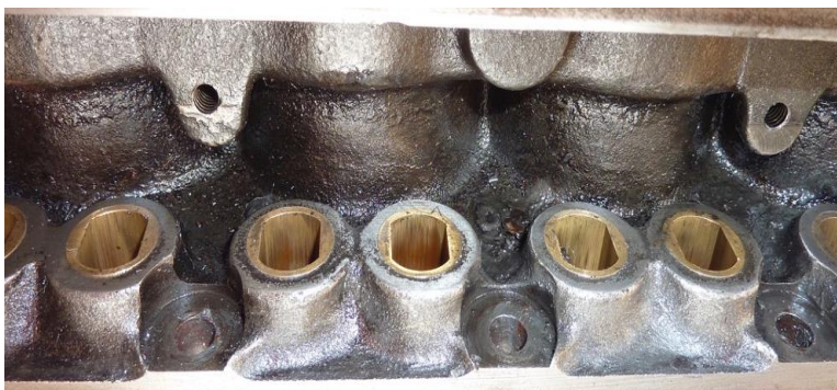
Machined tappet guides
