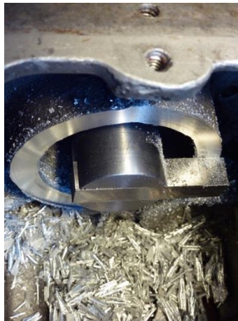
Flange being removed
