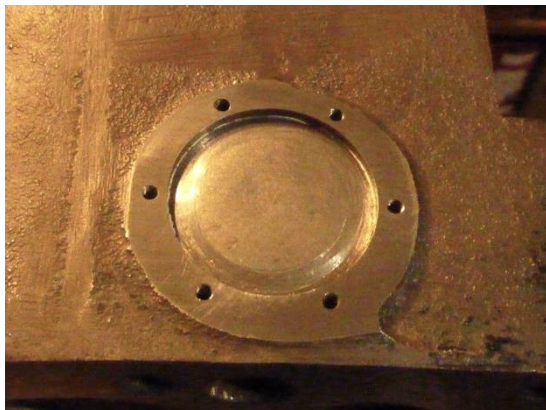
Plug fitted & 6BA holes tapped
