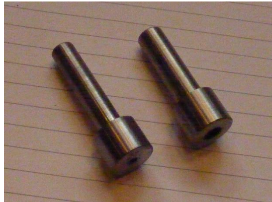
Two head stud drilling ferrules
