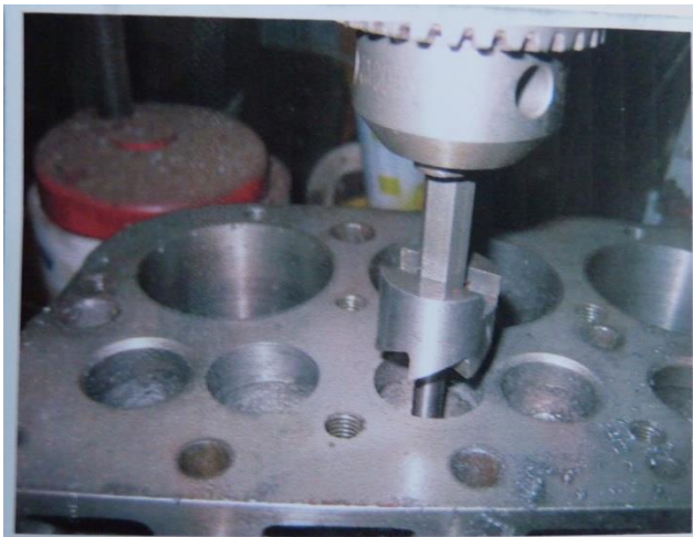
Boring for larger inlet valves
