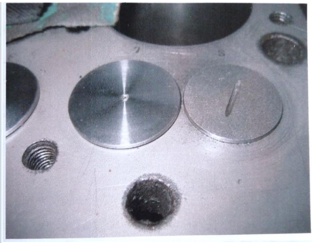
Large inlet valve in position
