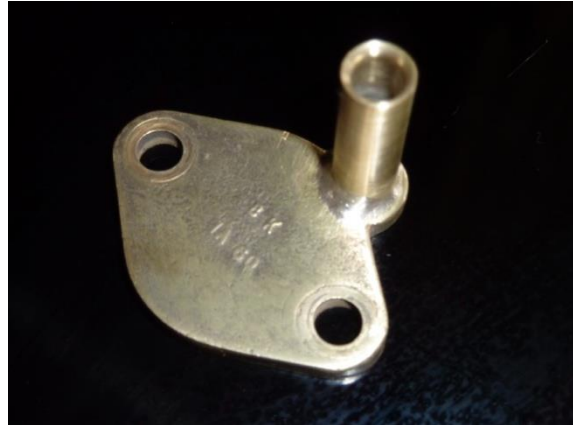
lengthened oil pump pick-up
