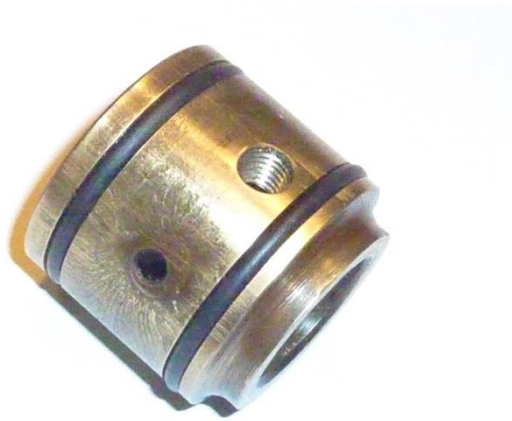
Front cam bearing ready for installation
